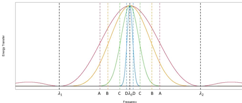
**Figure 7:** Energy transfer functions and KZFT filters centered at  $\lambda_0$  for parameters  $m$ , such that  $\frac{1}{m} = \lambda_0 - \lambda_1 = \lambda_2 - \lambda_0$  and  $k = 1$  in red with cut-off (A),  $k = 2$  in orange with cut-off (B),  $k = 10$  in green with cut-off (C),  $k = 100$  in blue with cut-off (D).
