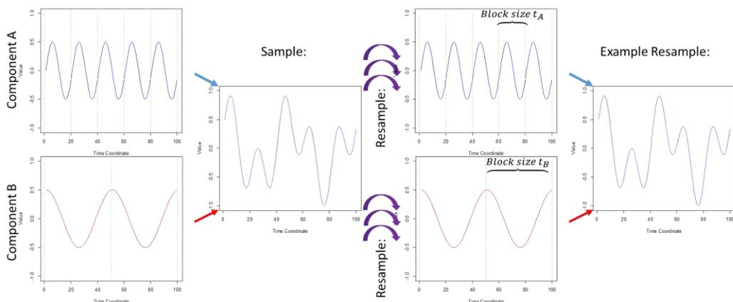
**Figure 5:** Illustration of resampling a MPC time series with PC component A of period,  $p_A$ , and a different PC component B of period,  $p_B$ . After PC component separation, the strategy incorporates the period,  $p_A$  and  $p_B$ , in the design of block length for block bootstrapping respectively, replicating the PC structure of component A and component B.
