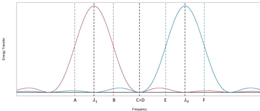
**Figure 8:** Illustration of the energy transfer functions from a KZFT filter centered at  $\lambda_1$  with cut-offs A and B and a KZFT filter centered at  $\lambda_2$  with cut-offs E and F. C and D are the frequencies excluded by the choice of window size in the respective KZFT filters, set here to be halfway between frequencies  $\lambda_1$  and  $\lambda_2$ .
