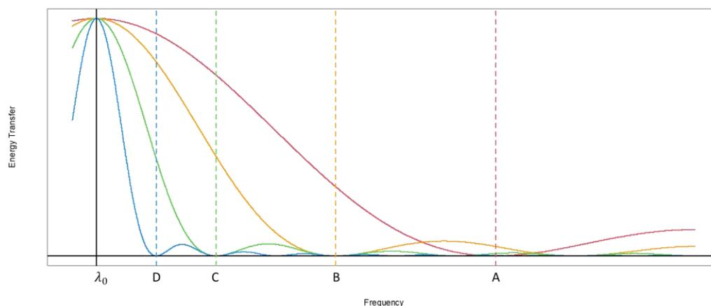
**Figure 6:** One side of the symmetry energy transfer functions for Kolmogorov-Zurbenko filters centered at frequency  $\lambda_0$  with parameters  $k = 1$  and A)  $m = 3$  in red, (B)  $m = 5$  in green, (C)  $m = 10$  in blue, and (D)  $m = 100$  in purple.
