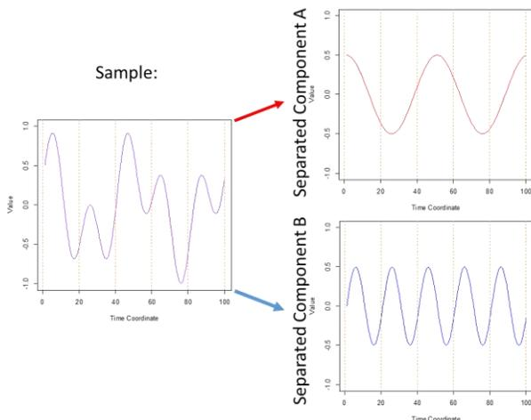
**Figure 4:** Illustration of separating a MPC time series into PC components
