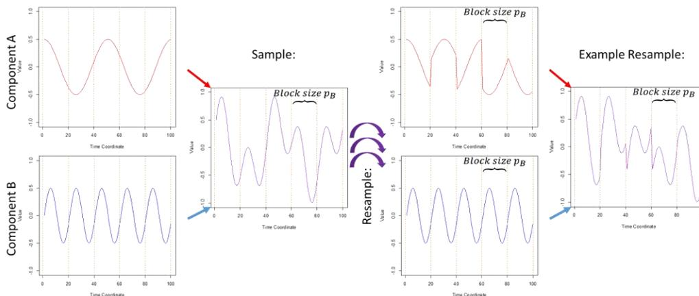
**Figure 3:** Illustration of resampling a MPC time series with PC component A of period,  $p_A$ , and a different PC component B of period,  $p_B$ , with a block bootstrapping strategy that incorporates the period,  $p_B$ , in the design of block length, replicating the PC structure of component B but failing to replicate the PC structure of component A.
