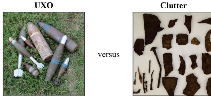
Figure 2: UXO (left) and metallic clutter objects (right) found near UXO on land. Reproduced from Cazares et al. (2021).
