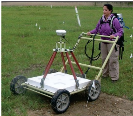
Time-domain Electromagnetic Multi-sensor Towed Array Detection System (TEMTADS), developed by the Naval Research Laboratory and Nova Research
