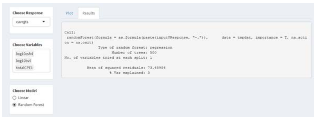
Figure 10: When a random forest is chosen, the Results page of the Modeling tab displays a summary of the model, including the number of trees and the mean of the squared residuals.
