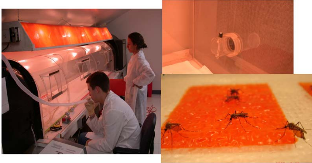
Figure 8: Left panel: wind tunnel. Air enters from the left and can be mixed with human breath or other gasses. Mosquitoes are released from the cannister at the right side of the tunnel (enlarged in the upper right panel). If they fly up-wind (to the left), they will encounter a feeding platform with warmed nutrient fluid under a membrane in several wells (one well is enlarged in the lower right panel). They may probe (pierce) the membrane and imbibe the nutrient liquid.
