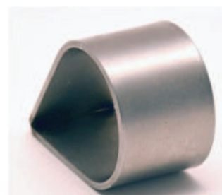
(c) Experimental “Teardrop” Used to Simulate the Stresses In the Container.
