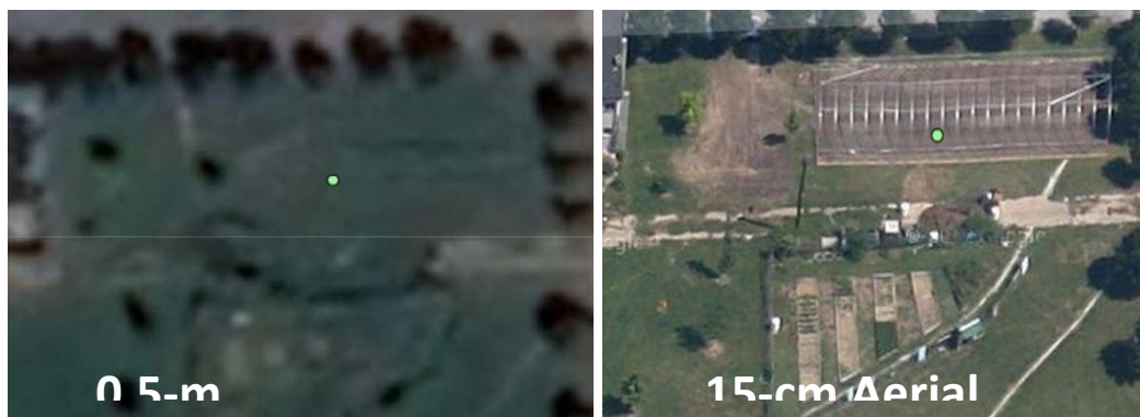
Figure 2: Comparison of an agricultural site using 0.5-m 2 satellite imagery (left) and 15-cm 2 aerial imagery (right). The green dots represent the same location in space.
