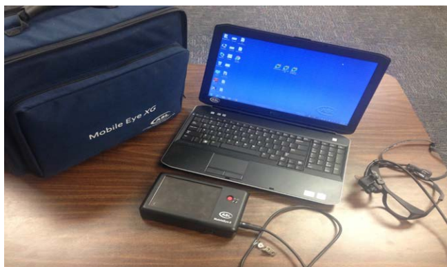
Figure 1: ASL mobile eye tracker equipment showing the DTU in the front, the eye tracking glasses to the right, and the laptop in the back.
