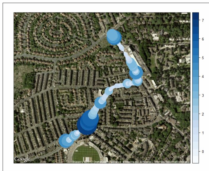
Figure 6: loa GoogleMap bubble plot visualization of vehicle CO 2 emissions. Mobile data was collected at 1-second resolution using a standard (EURO II petrol) passenger car and a Horiba OBS-1300 PEMS/GPS, and emissions reported in grams. Google Map data subject to copyright © 2012 Google/Terrametrics/GeoBais-DE/BKG/Tele Atlas.
