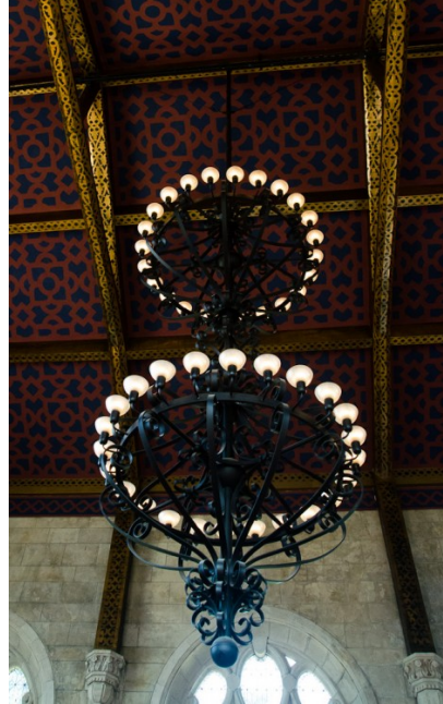
Figure 2. LED bulbs in this difficult to reach chandelier have not needed to be replaced in over a year. Previous generation bulbs burned out within two months [5].
